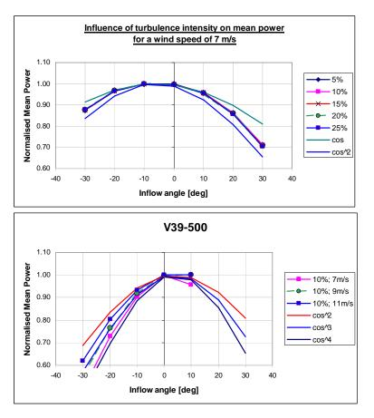
Figure 4-12. Normalised power of pitch regulated wind turbines simulated with PHATAS (upper) or GAST (lower) as function of inflow angle. The powers of the cosine dependency on the inflow angle are indicated additionally.
