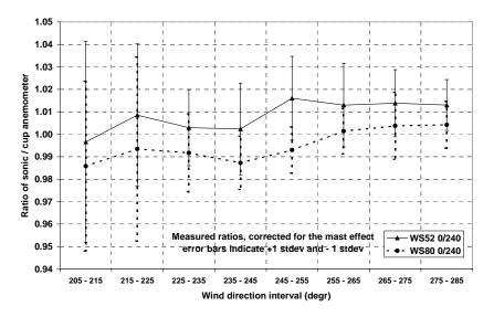
Figure 4-9 Ratios (corrected for mast and boom effects) between the Gill Wind Master sonic anemometer (0° boom direction) and the cup anemometer (240° boom direction) at 52m and at 80m, including the  $+1\sigma$  and  $-1\sigma$  error bars.
