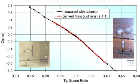
Torque measurements on Risoe P2546a cup anemometer @ 8 m/s
