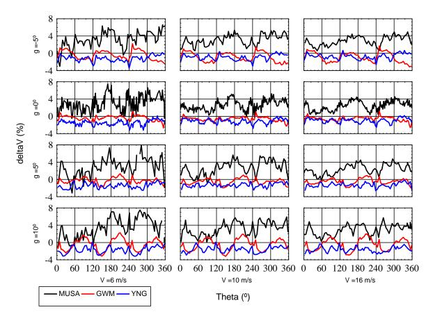
Figure 4-8 Results for the percentage deviation in the measurement of the total wind speed as function of the true wind direction relative to the sensor for four inclination angles and three wind speeds. DEWI wind tunnel.
