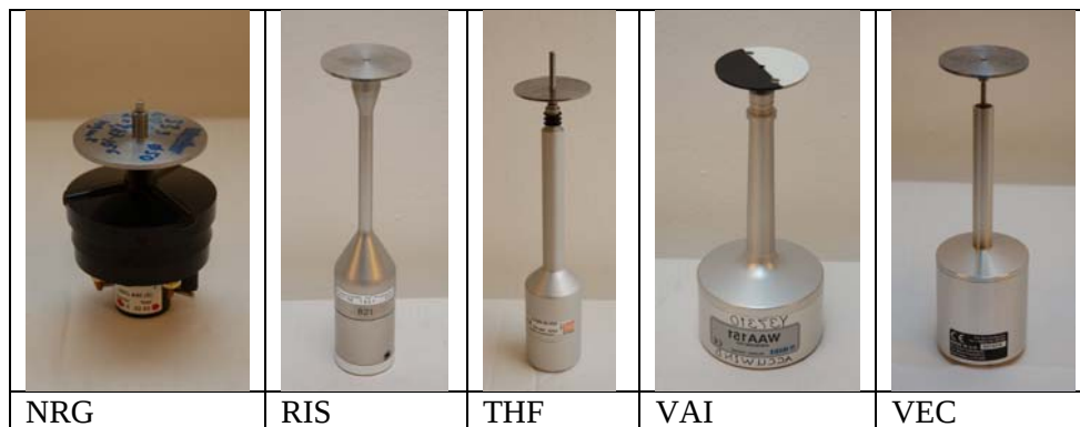
Figure 3-37 Flywheels mounted on cup anemometer shafts for flywheel deceleration tests in climate chamber according to the procedure in ref. 1.
