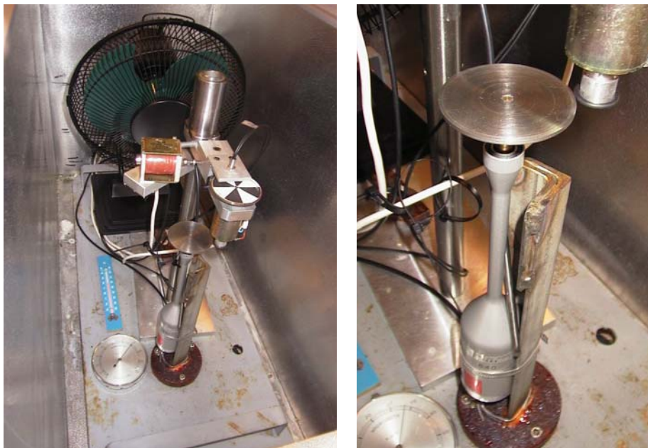
Figure 3-36 Bearing friction measurement setup in climate chamber. At left heater, fan, sensors, excitation mechanism, and the mounting of the cup anemometer with the flywheel is show. At right the flywheel and the driving motor is shown in detail.
