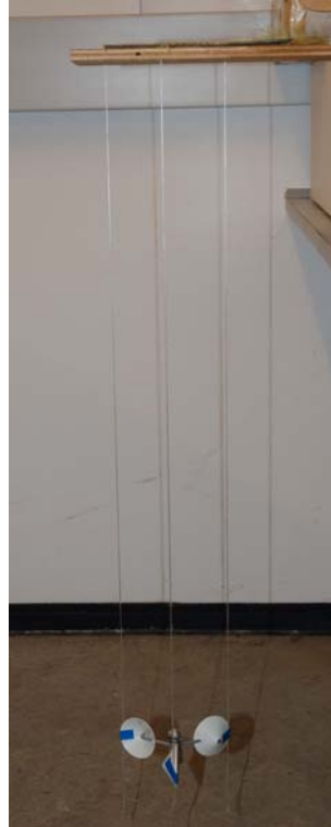
Figure 3-42 Determination of moment of inertia by oscillations of a Vector cup anemometer rotor. Length of strings 0.8m.
