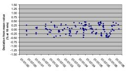
Figure 3. Results from Reference anemometer calibrations.
