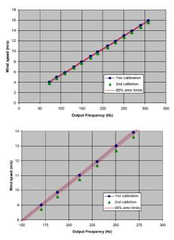
Figure 6. Recalibration results – unit with bearing damage, 15 months of operation on site a: full calibration scale b: detail
