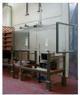
Figure 2. CRES wind tunnel.
