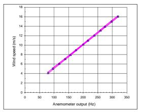
Figure 4 Response characteristics of a VECTOR A100K cup anemometer with calibration error limits (typical error 95%)
