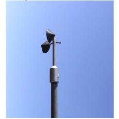
Figure 1. Anemometer damaged from lightning strike
