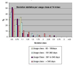
c: Reference wind speed 14 m/s Figure 9. Distribution of recalibrations per deviation class
