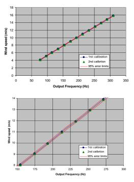
Figure 5. Recalibration results – undamaged unit, 15 months of operation on site a: full calibration scale b: detail 95% error limits correspond to the 1rst calibration
